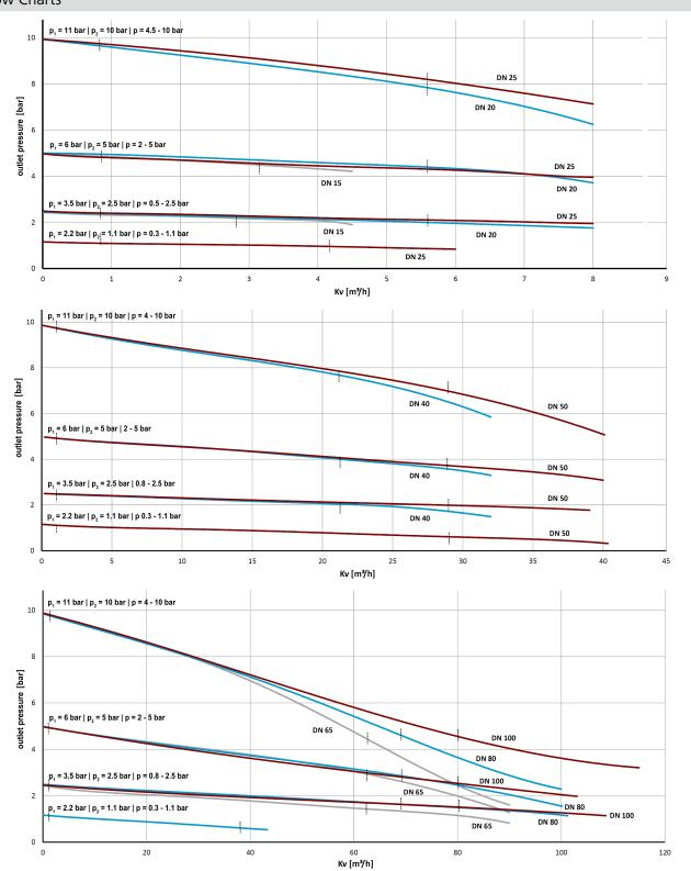
$p = pressure \ \ \, p_1 = inlet \ pressure \ \ \, p_2 = adjusted \ outlet \ pressure \ \ \, i = recommended \ working \ range$
